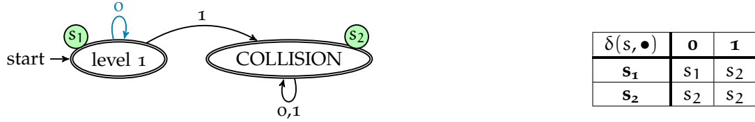
Figure 3.20: Automaton 4: Level 1. On the right, transition function which represents it.
