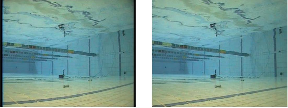
**Figure 4.3:** Left, a frame from a video recorded in an underwater environment. Right, the same frame after undistortion.
