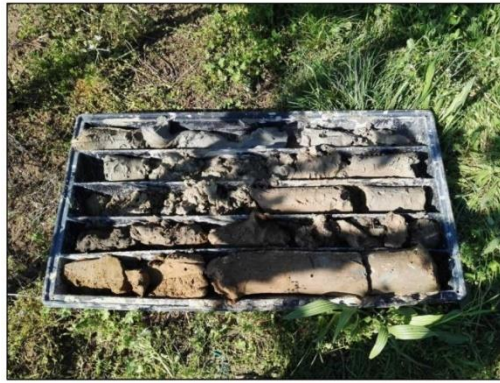
Photo 3.10. S4 Survey samples from 5 to 10 m (GEOLAMBDA Engineering S.r.l.,2018)
