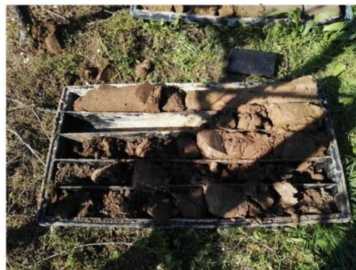
Photo 3.9. S4 Survey samples from 0 to 5 m (GEOLAMBDA Engineering S.r.l.,2018)
