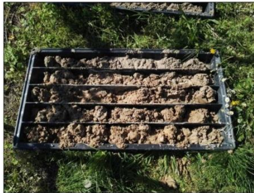
Photo 3.3. S1 survey Samples from 5 to 10 m (GEOLAMBDA Engineering S.r.l.,2018)
