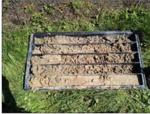
Photo 3.6. S2 Survey samples from 5 to 10 m (GEOLAMBDA Engineering S.r.l.,2018)
