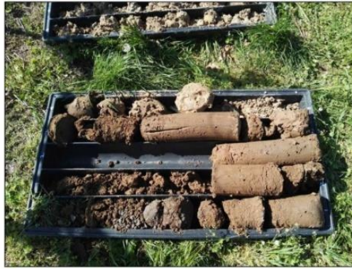
Photo 3.2. S1 survey Samples from 0 to 5 m (GEOLAMBDA Engineering S.r.l.,2018)
