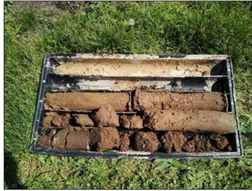
Photo 3.14. S7 Survey samples from 0 to 3 m (GEOLAMBDA Engineering S.r.l.,2018)
