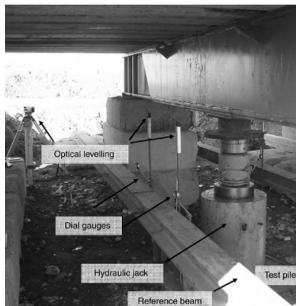
Figure 1.16. Dial gauges for measuring pile head settlement (Viggiani & al., 2012)
