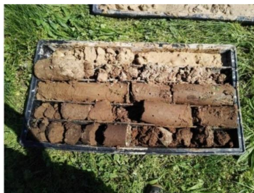
Photo 3.5. S2 Survey samples from 0 to 5 m (GEOLAMBDA Engineering S.r.l.,2018)
