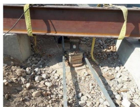
Test n.3- detail of jack and sensor positioning
