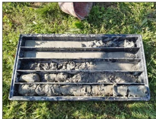
Photo 3.11. S4 Survey samples from 10 to 15 m (GEOLAMBDA Engineering S.r.l.,2018)
