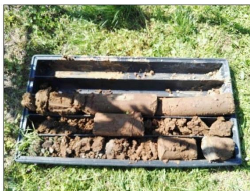
Photo 3.12. S5 Survey samples from 0 to 3 m (GEOLAMBDA Engineering S.r.l.,2018)
