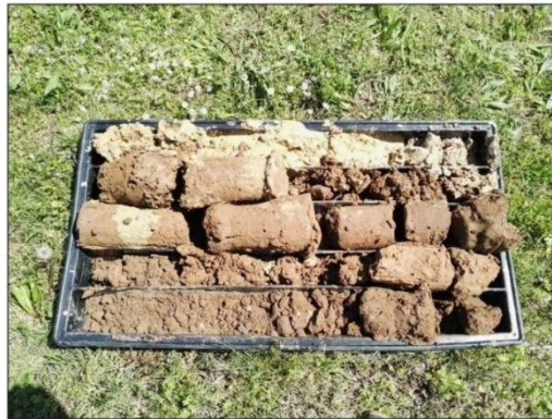
Photo 3.7. S3 Survey samples from 0 to 5 m (GEOLAMBDA Engineering S.r.l.,2018)
