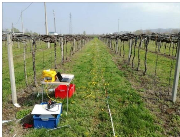
Photo 3.15. View of the MASW spreading carried out (GEOLAMBDA Engineering S.r.l.,2018)
