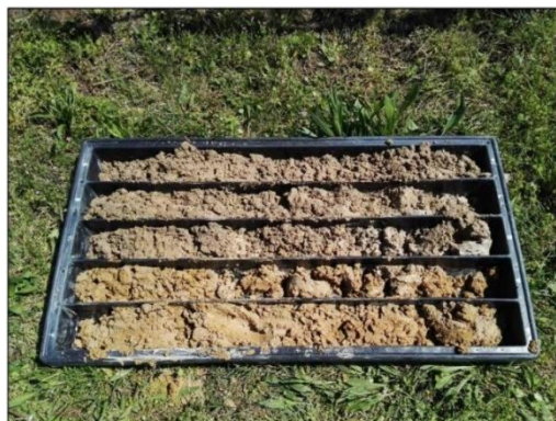
Photo 3.8. S3 Survey samples from 5 to 10 m (GEOLAMBDA Engineering S.r.l.,2018)
