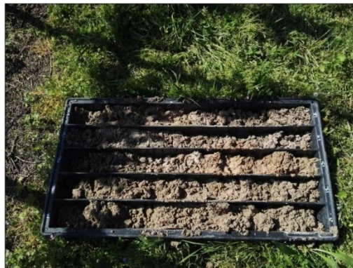
Photo 3.4. S1 survey Samples from 10 to 15 m (GEOLAMBDA Engineering S.r.l.,2018)
