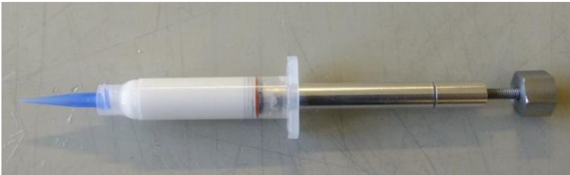
Figure 8. 5mL syringe with attached pin of 410 \mu\text{m}
