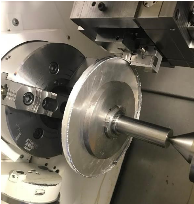
Figure 51: Aluminium workpiece destroyed
