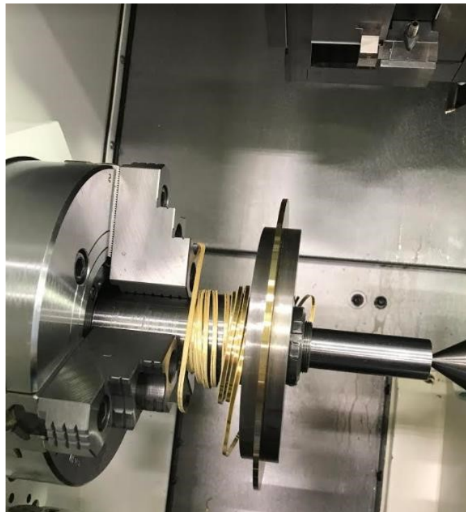
Figure 54: Rolling of the extruded chip on the spindle.
