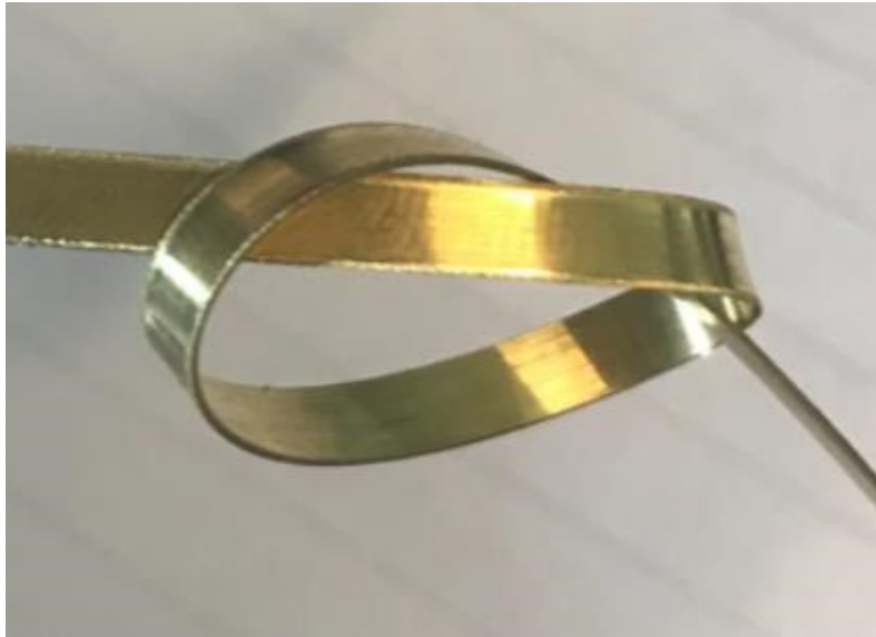
Figure 10: The ductility of a brass strip from extrusion cutting.
