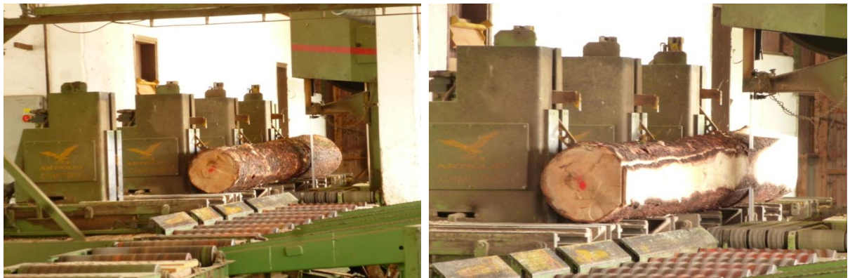
Figure 3.8| (a and b) The band saw cutting the trunks in raw boards.
