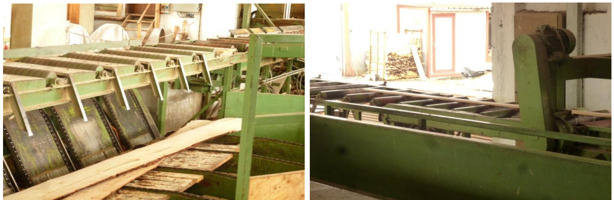
Figure 3.9| (a) Detail of the belt conveyors system and (b) finished boards exiting the trimmer.
