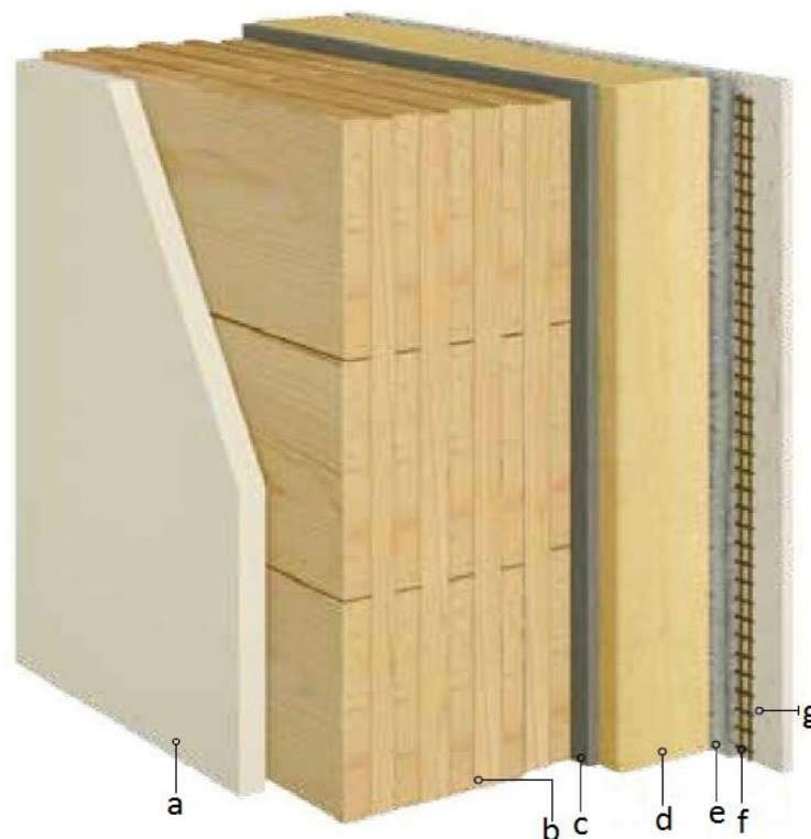
Figure 3.3| Section of the chosen type of MHM wall.3.1.4. Brick wall product system
