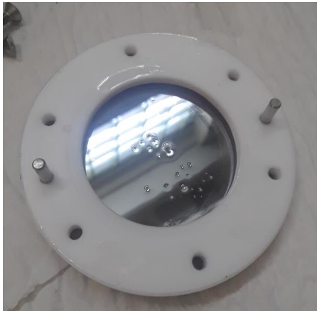
Figure 7.23: Disassembled chamber after Meniscus test 11 with dust particles in octane pool
