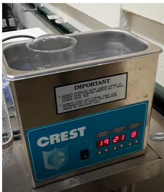
Figure 4.3: Ultrasonic cleaning machine during a cleaning process
