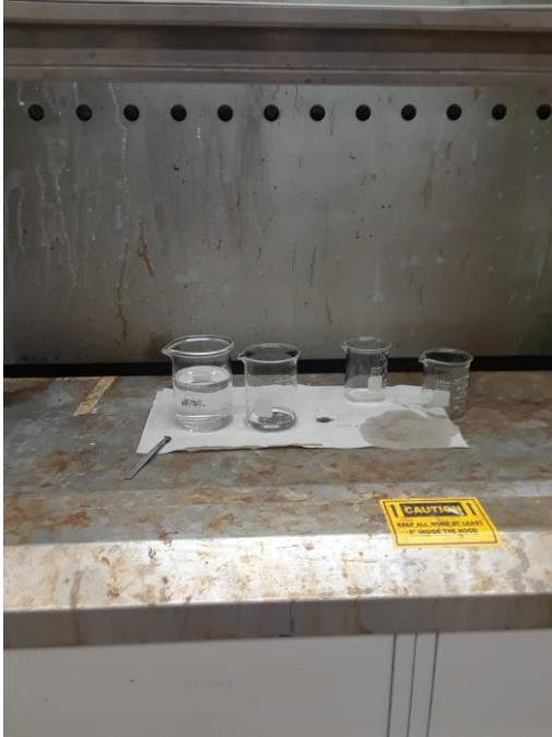
Figure 4.1: Glass beakers under the fume hood during piranha cleaning process (left); silicon wafer bathed in piranha mixture (right)
