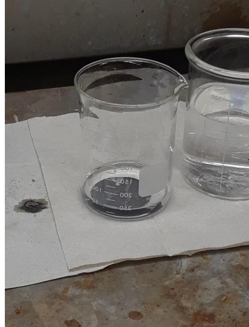
Figure 4.1: Glass beakers under the fume hood during piranha cleaning process (left); silicon wafer bathed in piranha mixture (right)
