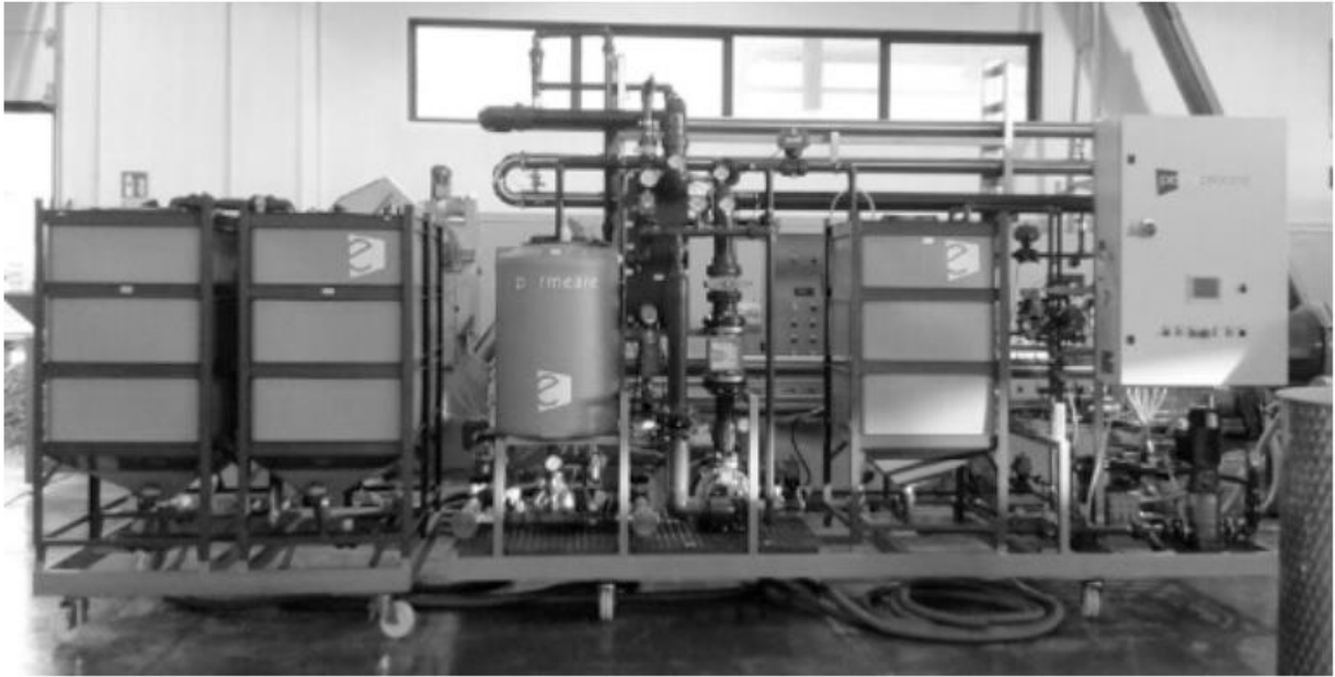
Figure 10: Filtration treatment of OMWW machine (La Scalia Giada 2017)
