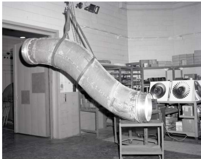
FIGURE 1.1: S-duct in the engine research building.
