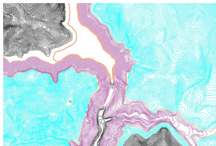
Figure 4.1.3: Modified contour lines without dam and water in the reservoir
