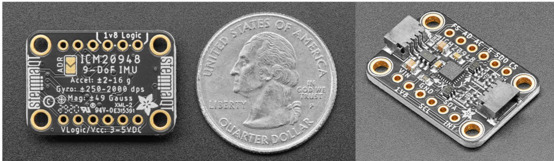
Figure 5.2: Back and front view of an Adafruit TDK InvenSense ICM-20948 9-DoF IMU
