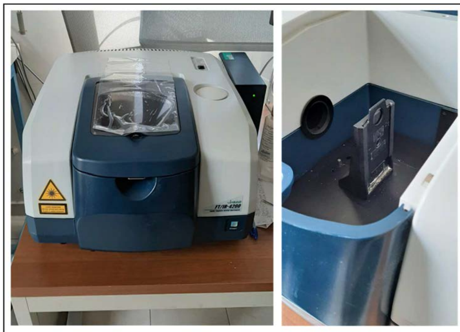
Figure 2.28 Jasco FT/IR 4200 spectrometer (left) and sample holder for KBr disks.
