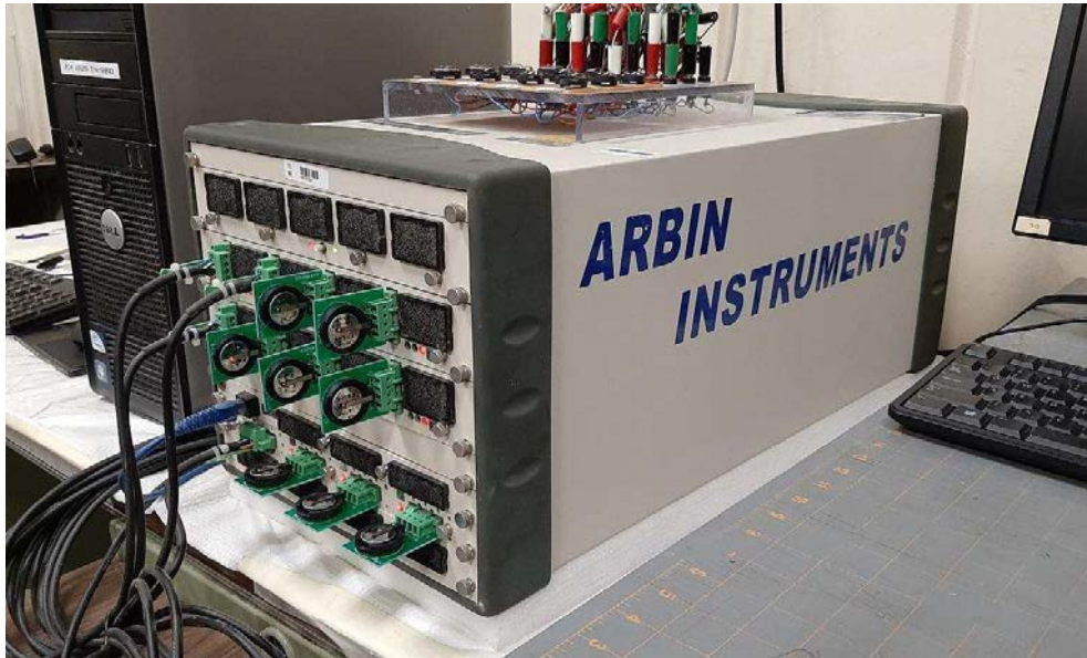
Figure 3.4 Arbin Instrument BT-2000 battery test device
