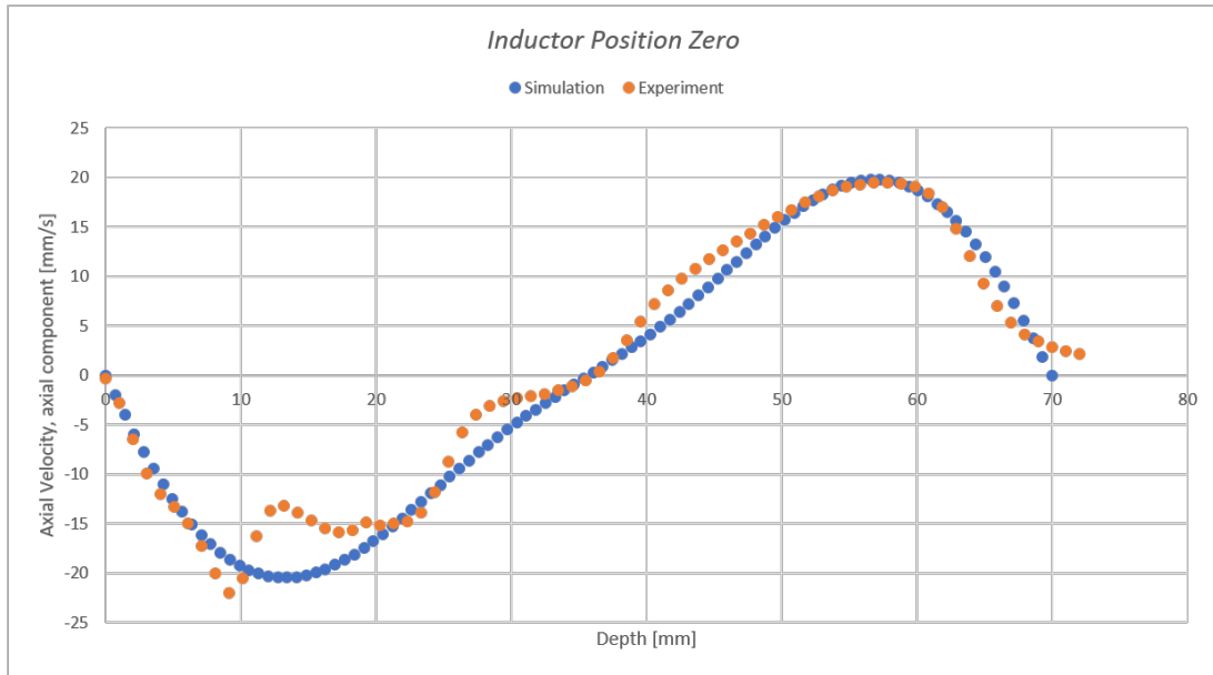
Fig. 3.22: Comparison between simulated and measured axial. Inductor Position Zero . Experiment maximum measured velocity: 22.04 [mm/s]; simulation maximum velocity: 20.47 [mm/s].
