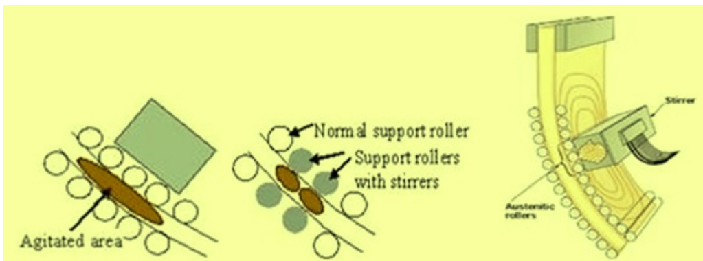
Fig. 1.11: Strand electromagnetic stirrer: location and design
