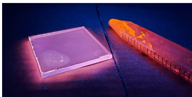
Figure 3.12 5.0 \times 5.0 \text{ cm}^2 PMMA film containing [\text{Eu}_2(\text{AFF})_4](\text{NEt}_4)_2 at the 0.9% by weight, showing anomalous pink emission under UV illumination at 365 nm (left), and red-emitting solid state sample of the same complex (right).
