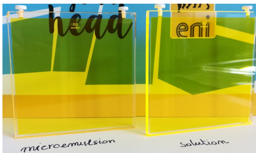
Figure 1.9 Cuvettes filled with a O/W microemulsion and a toluene solution of a completely water-insoluble organic dye, displaying unaltered optical transparency 38 .
