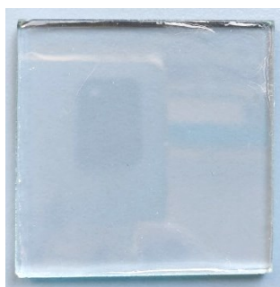
Figure 3.8 PMMA film of \sim 130 \mu\text{m} thickness, casted onto a 5.0 \times 5.0 \text{ cm}^2 treated glass slide and retaining initial adherence.
