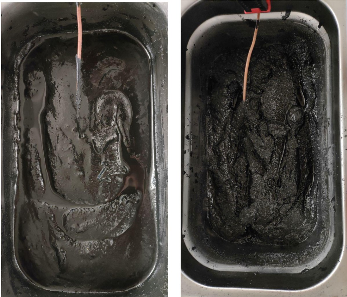
Fig. 7.9 - different consistency with 1% and 3% of graphene
