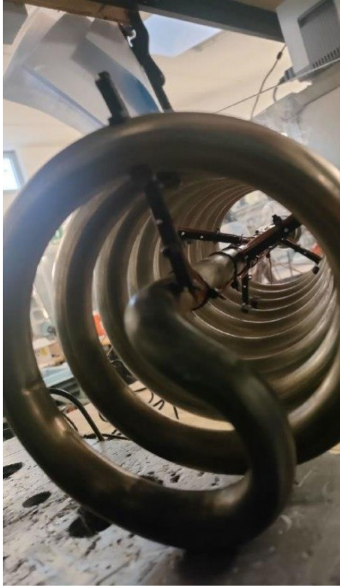
Fig. 3.6 & 3.7 - inside and outside view of supports in helix pipe
