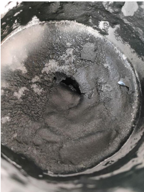
Fig. 8.3.1 & 8.3.2 - appearance of the solid paraffin surface
