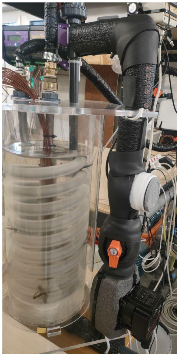
Fig. 2.5 - Thermally insulated external circuit
