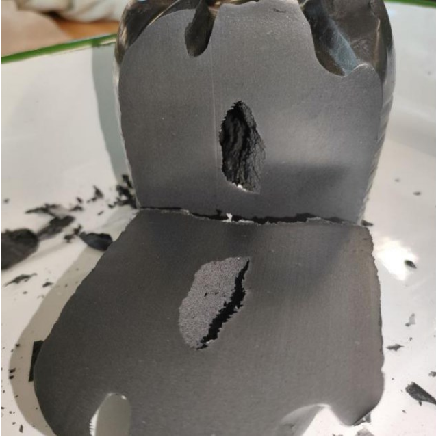
Fig. 8.3.3 & 8.3.4 - presence of voids inside the solid paraffin
