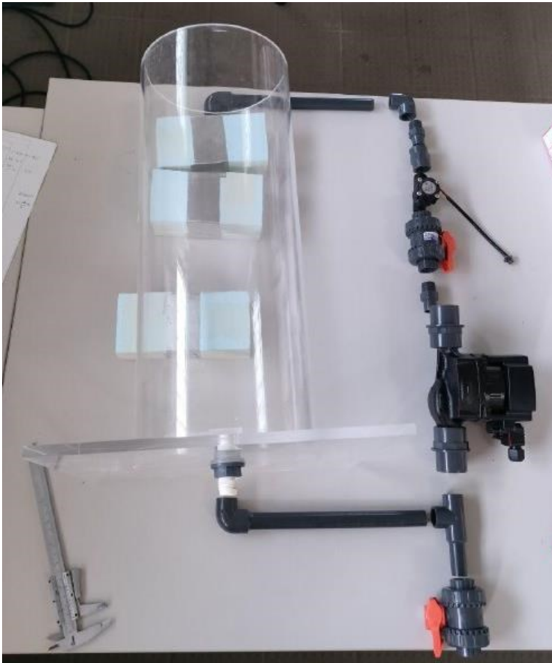
Fig. 2.3 - First investigation of the setup for the external circuit
