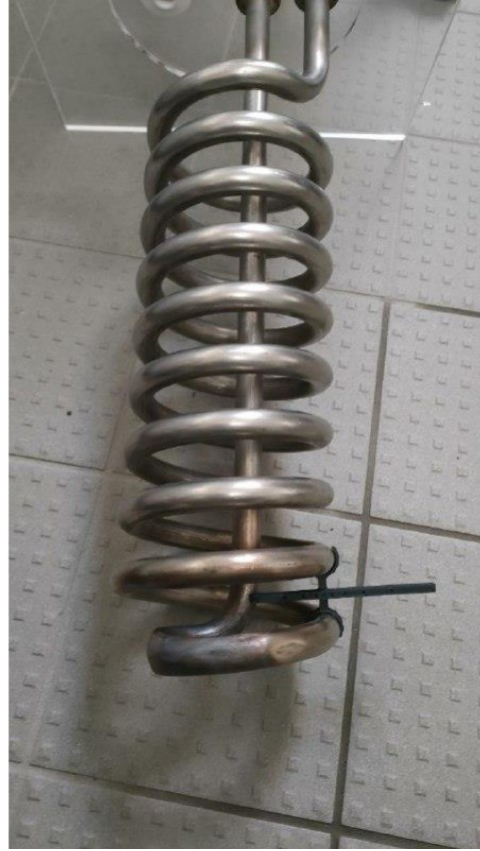
Fig. 3.6 & 3.7 - inside and outside view of supports in helix pipe
