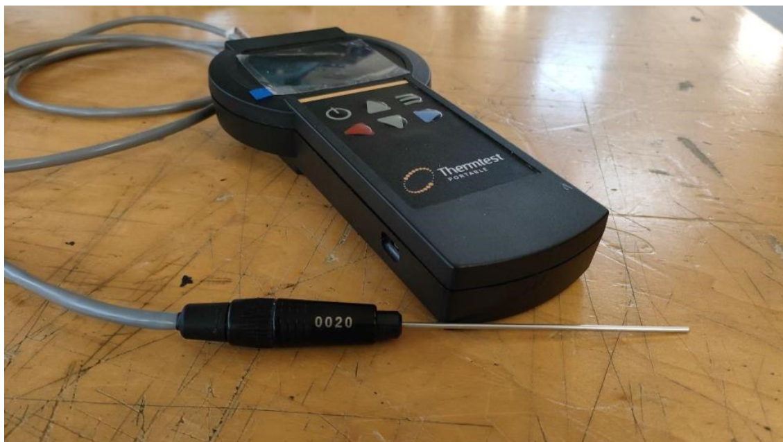
Fig 7.5 – Thermtest MP-2 with TLS 150 mm sensor
