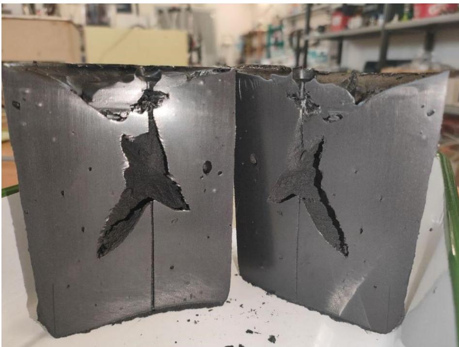
Fig. 9.1 - void created in solidification
