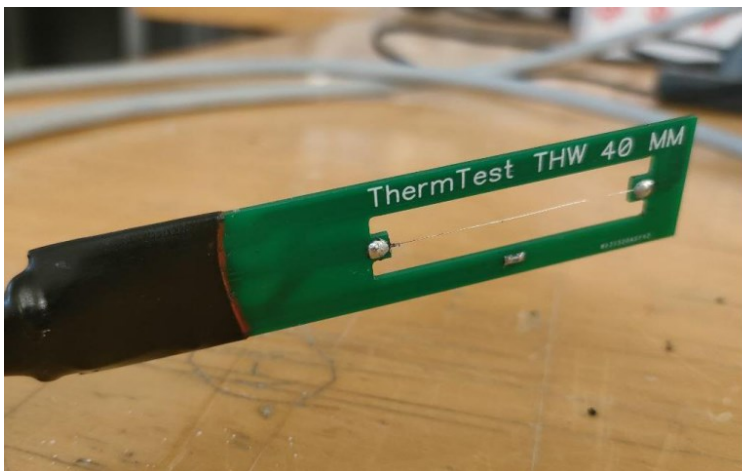
Fig. 7.3 & 7.4 - instrument for thermal conductivity measurement
