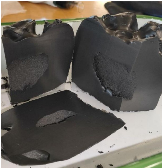
Fig. 8.3.5 & 8.3.6 - presence of voids inside the solid paraffin
