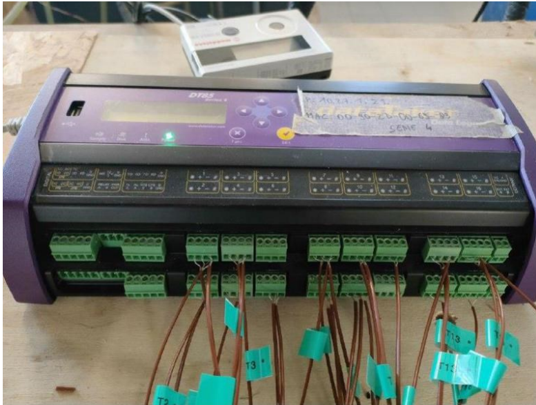
Fig 2.6 - Datalogger DT80 acquisition system
