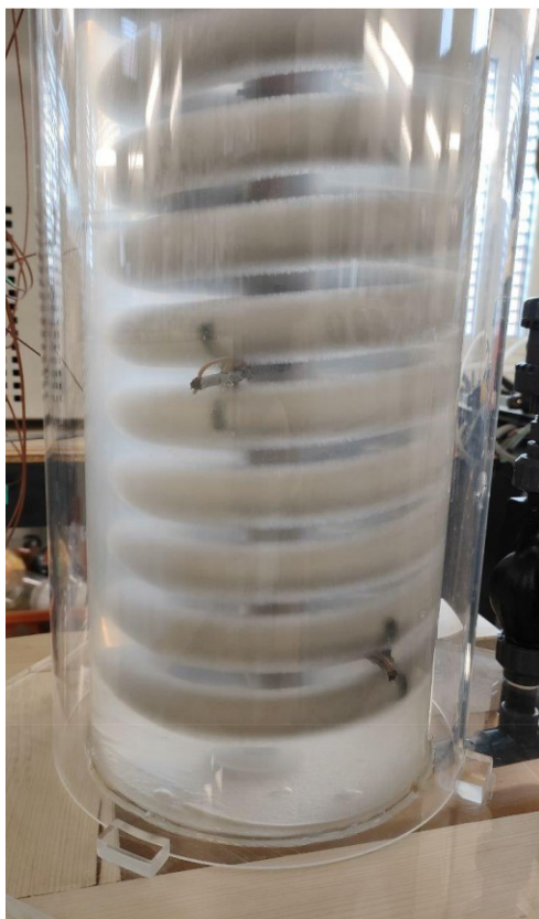
Fig.5.1.2 & 5.1.3 - solidification beginning and completed solidification with clear volume reduction
