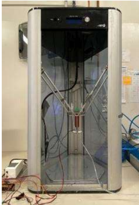
Figure 2.1. Image of 3D printer, Delta Turbo 2, WASP with the hybrid setup installed.
