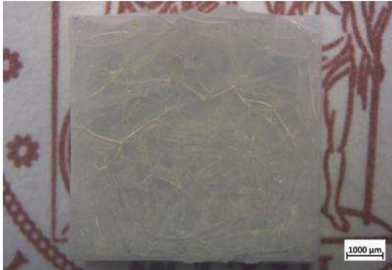
Figure 3.12. A sample of composition 1 of Lanthanum ink after sintering at 1350°C for 30 min.
