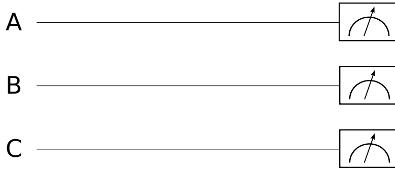
Figure 5.1.: Scheme of a trivial circuit where the three observers Alice , Bob and Charlie , referred respectively as A, B and C at the left of the circuit, are associated to a different communication channel (or equivalently, Hilbert space) and where no interaction is present between the channels. The measurement on the channels operated by the observer is represented on the right by the measurement box.
