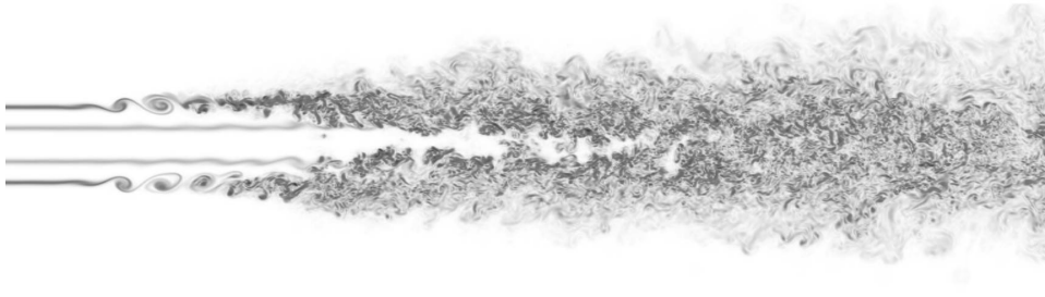
Figure 1.2: Example of a transition to turbulence in a subsonic co-axial jet flow (Prof. Dr. L.Kleiser).
