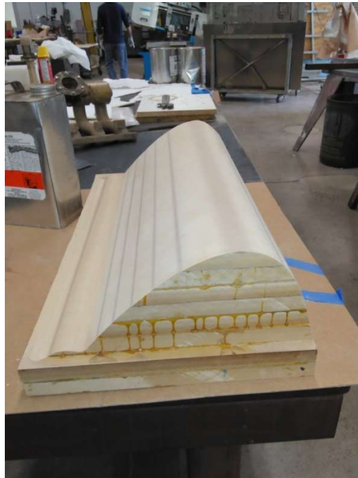
Figure 4.13 - Mold after sanding process
