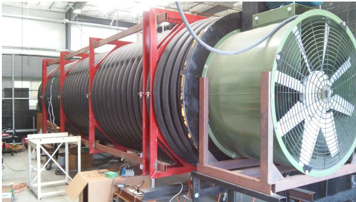
Figure 4.2 – Wind tunnel's structure and fan
