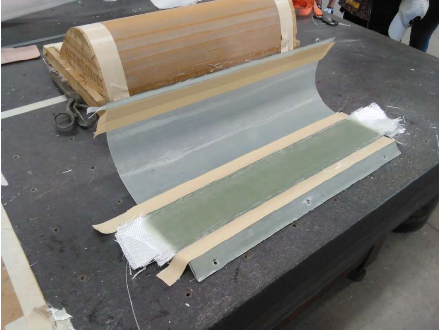
Figure 4.20 - Additional spread material for the increase of the weight and to reinforce the tips
