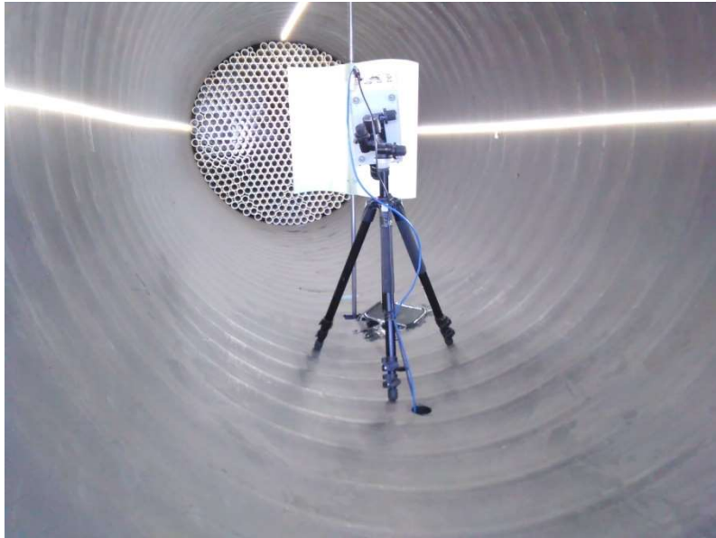
Figure 5.1 - High speed camera placed in the tunnel focusing the reflected image on the mirror
