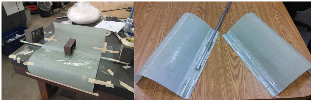
Figure 4.15 - Squeezed blades to mold the shaft location (left), the shaft location obtained and drilled (right)
