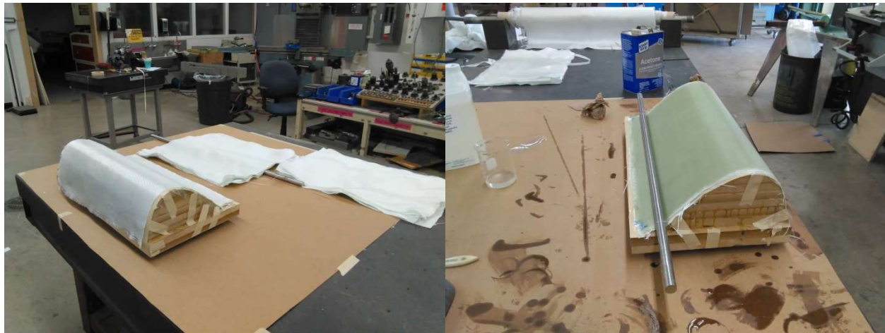
Figure 4.14 - First fiber layer spread on the mold (left) and the blade after 6 layer of fiberglass with a sample of the real shaft pressed on its location to preserve a good semicircular shape (right)
