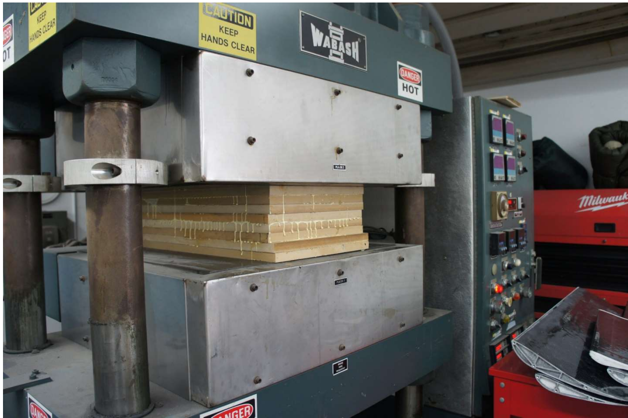
Figure 4.11 - Press used to help to stick the mold's wood layers
