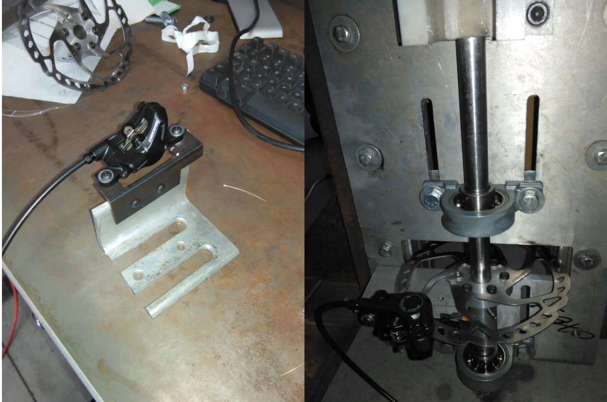
Figure 4.6 – Brake support (left), brake mounted on the test stand (right)
