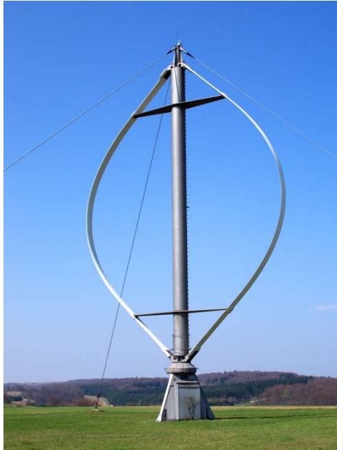
Figure 1.10 - Classic Darrieus rotor (Source: [49])
