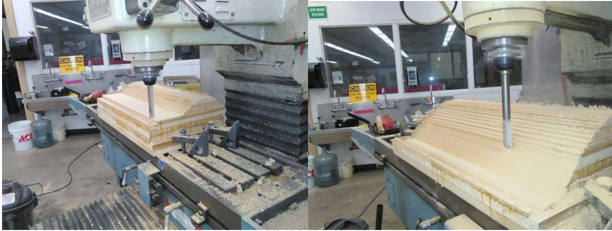
Figure 4.12 - Preliminary rough removal of material from the mold (left) and real precise shape cut (right)
