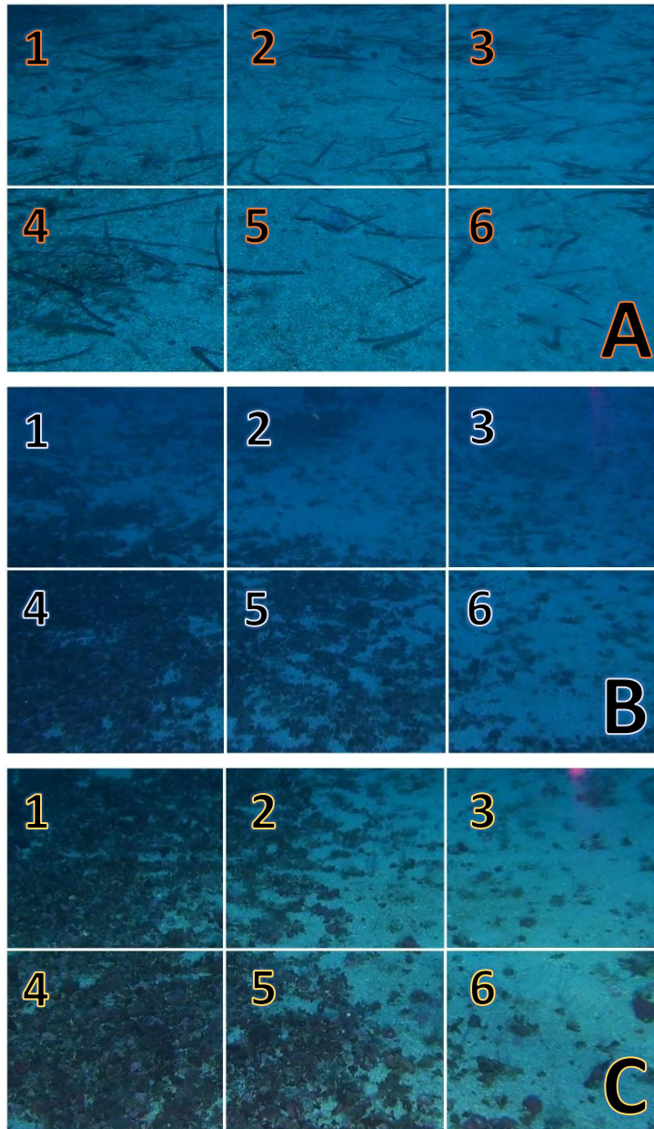
Figure 10. Visual representation of the grid system method, used for the ROV images' coverage calculation. By adding together, the separated parts own coverages, the entire coverage on the frame can be calculated more precisely. The segment A/6 contains 100% bioclastic sand, on the segment B/4 rhodolith is covering 90% of the substrate, while on the segment C/5 this number is around 60%, etc. The final coverages on the images became: (A) 90% bioclastic sand - 10% rhodolith; (B) 65% fine unconsolidated substrate - 35% rhodolith; (C) 55% bioclastic sand - 45% rhodolith. While these numbers can be estimated only approximately, this method is adequate enough to decide which is the dominating substrate and habitat on the given image.
