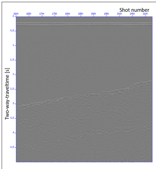
Figure 3.15: Zoom on common offset class 1 with filter 15-30-40-80 Hz.
