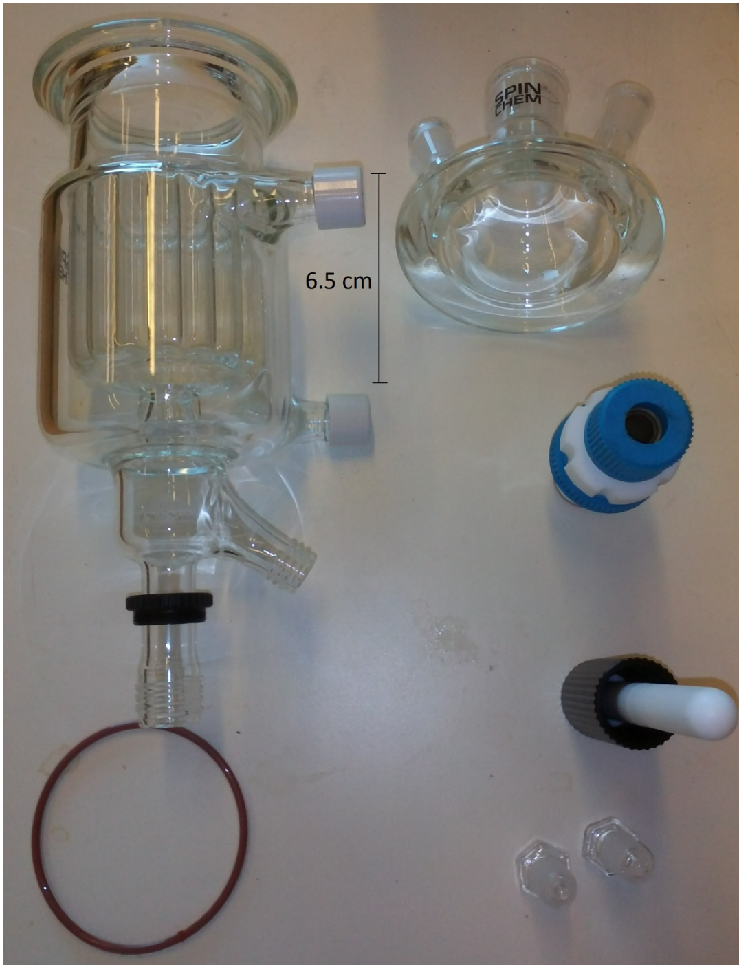
Figure 2.18 The vessel V211, the lid, the specific plug, the coated seal and the rod.
