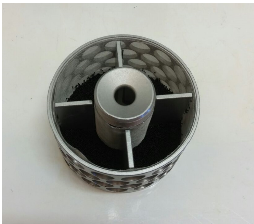
Figure 2.27 The solid catalyst Amberlite IRN 99 inside the SpinChem® RBR S221
