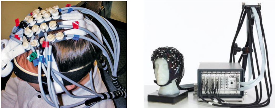
Figure 1.1: left: typical adult probe placement during an fNIRS acquisition. Blue and red flags display sources and detectors respectively. The gray cables are the optical fibers. (Taken from [46]). Right: an example of an fNIRS instrumentation (taken from [47]).
