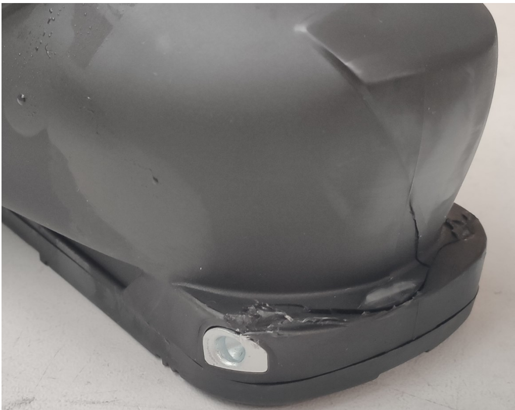
Figure D.4: Grilamid shell broken during test number 3, performed with an impact energy of 236.2 joules
