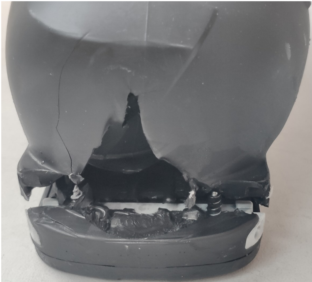
Figure D.5: Grilamid shell broken during test number 4, performed with an impact energy of 216.7 joules
