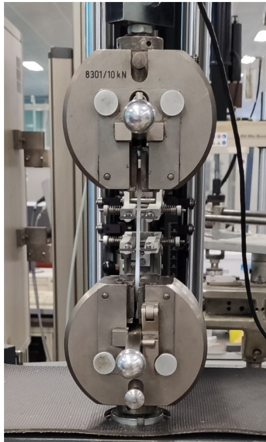
Figure 6.6: tensile tests at high strain rates in the company's traction machine
