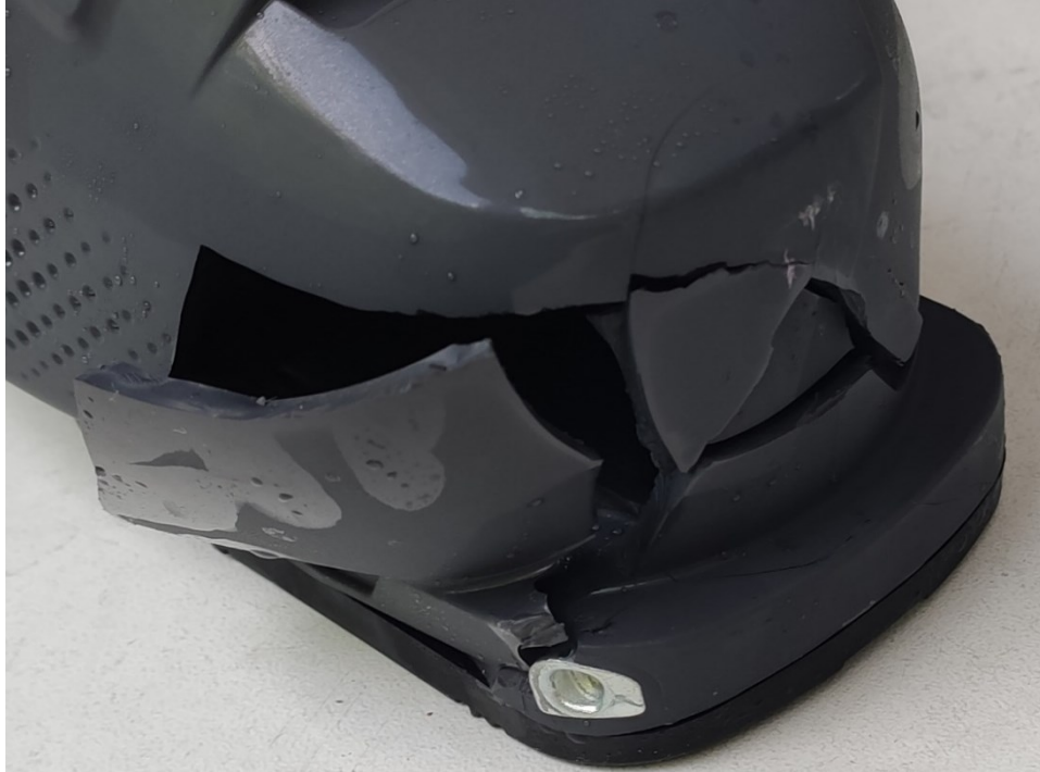
Figure D.1: Laripur shell broken during test number 2, performed with an impact energy of 99.3 joules
