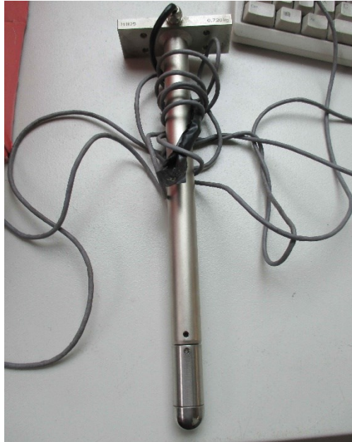
Figure 5.10: instrumented stem of Fractovis drop test machine
