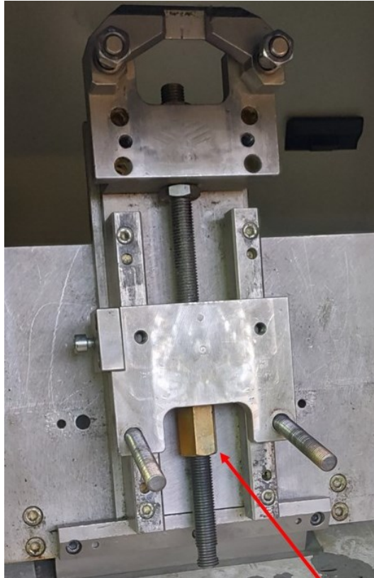
Figure 5.4: brackets that fix the tip and heel of the shell for the impact test; the red arrow indicates the screw that allows the distance between the two brackets to be adjusted to suit the length of the shell
