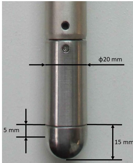
Figure 5.11: dimensions of the end of the instrumented stem
