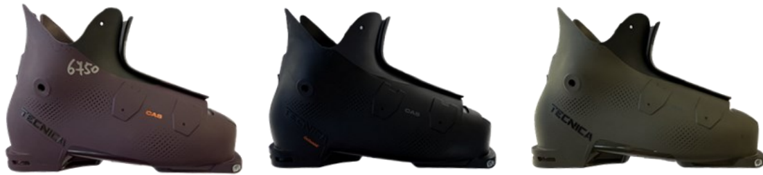
Figures 1.6-1.7-1.8: Markab shells in Laripur (purple), Grilamid (black) and Elastollan (green)
