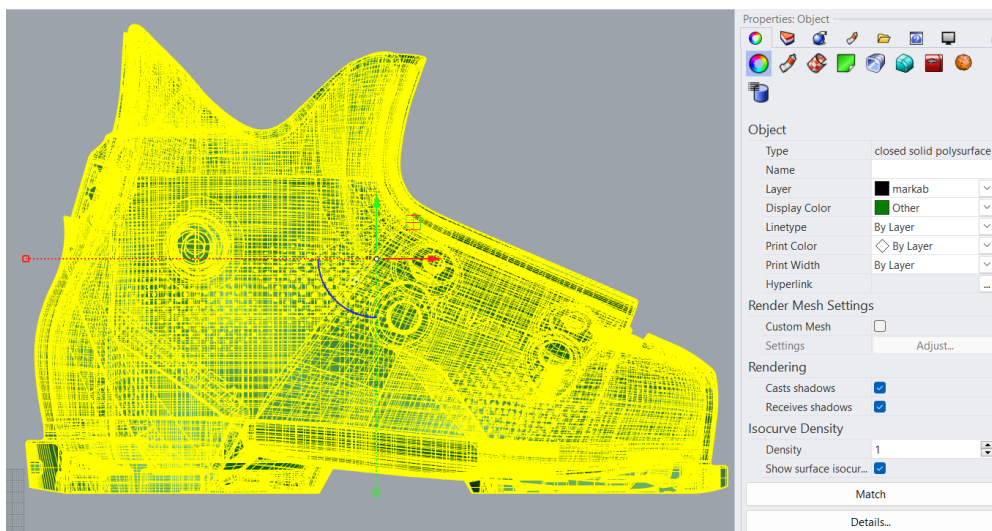
Figure 2.30: after correcting all the naked edges, the boot shell geometry results in a 'closed solid polysurface'
