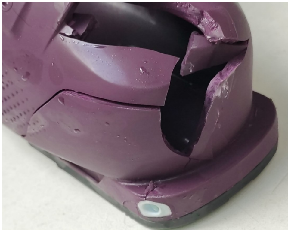
Figure D.2: Laripur shell broken during test number 5, performed with an impact energy of 94.2 joules
