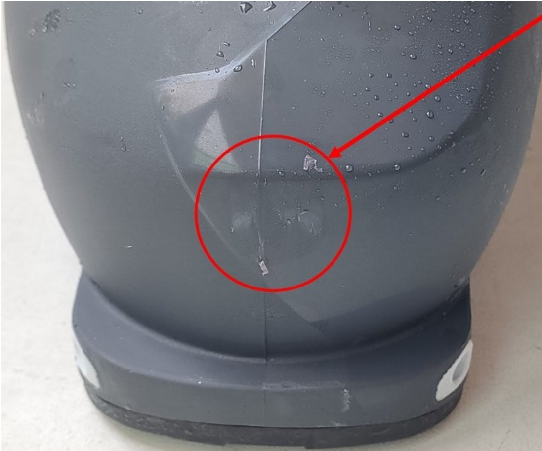
Figure 5.23: mark left by the impactor on the tip of the Laripur shell in test number 4
