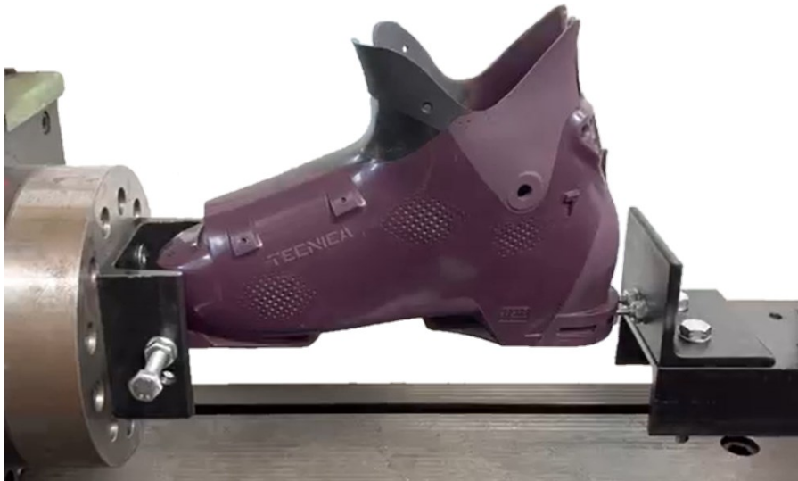
Figure 3.15: Laripur shell mounted on ski touring binding configuration
