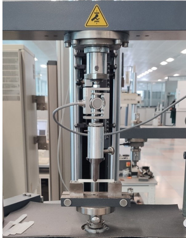
Figure 4.41: testing machine used in the company for the three-point bending test
