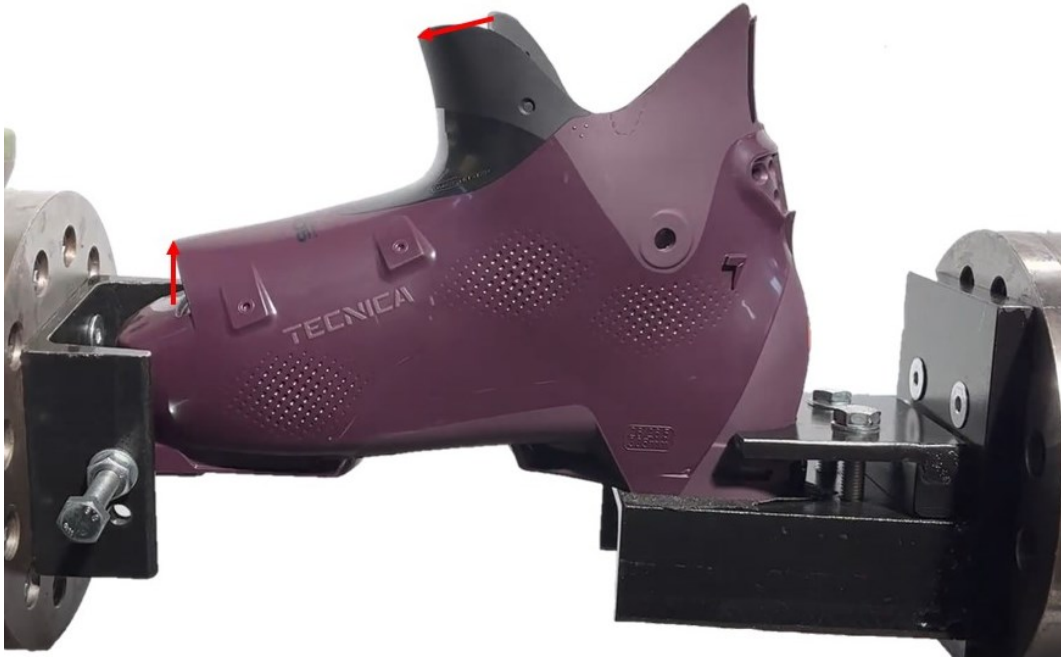
Figures 3.19: Laripur shell deformation for a rotation of ten degrees when the hybrid ski binding configuration is applied
