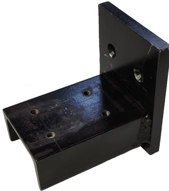
Figure 3.4: welded structure consisting of the vertical plate and the c-beam
