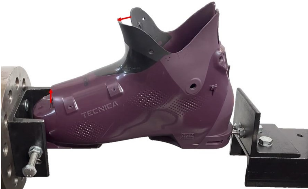
Figure 3.20: deformation of the Laripur shell for a rotation of ten degrees when the hybrid ski touring binding configuration is applied; as can be seen with the help of the arrows, the shell deformation is less than with the hybrid configuration of ski bindings ( figure 3.18 )
