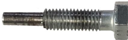
Figure 3.7: geometry of the screws used to simulate the posterior ski touring pins
