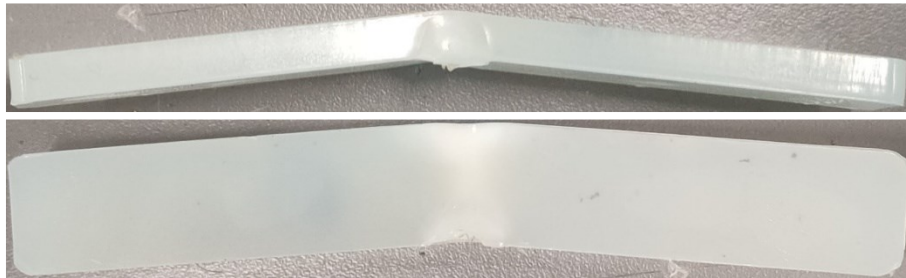
Figures 6.2-6.3: specimen plastically deformed but intact as a result of a Charpy impact test in which the hammer hit it on the 4 \text{ millimetres} thick side
