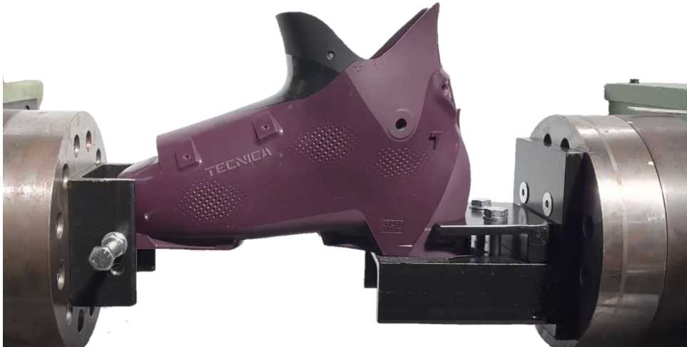
Figure 3.8: Laripur shell mounted on hybrid ski binding configuration
