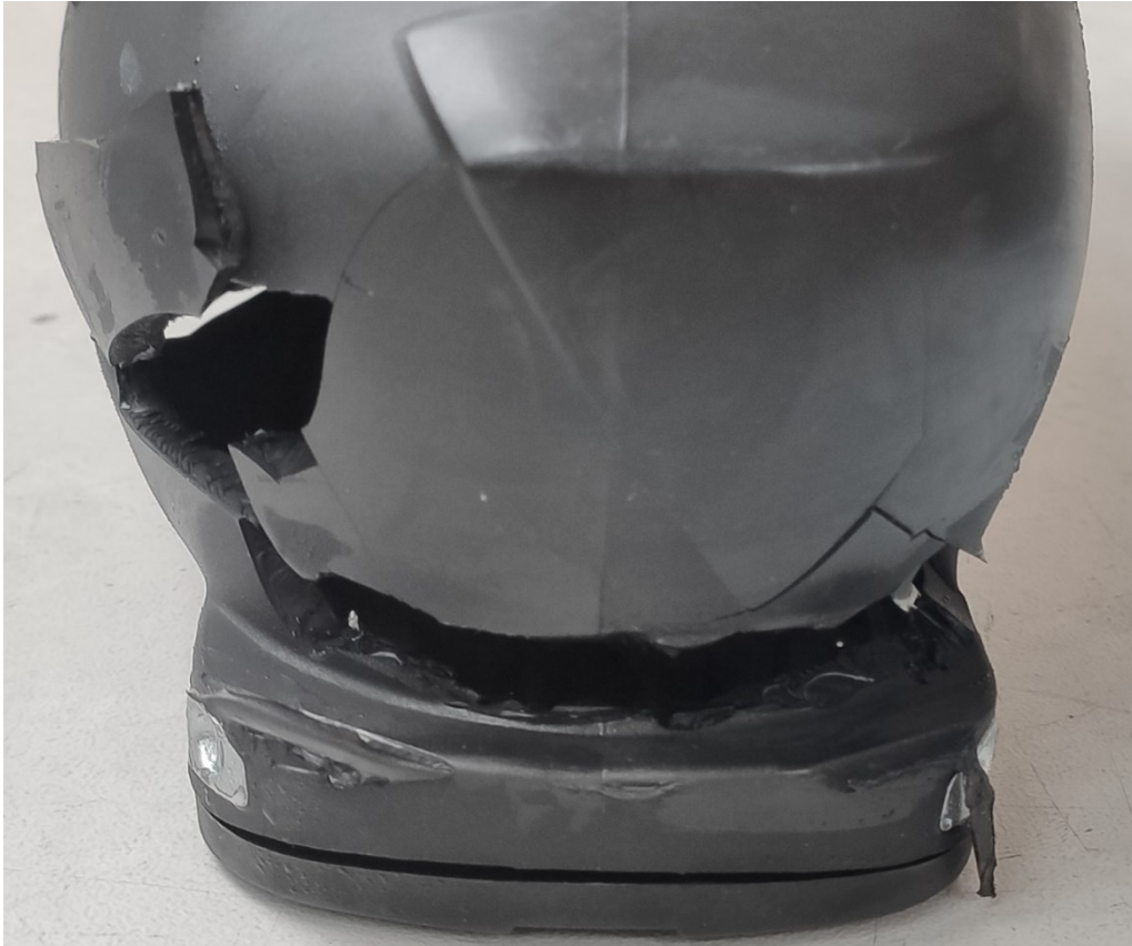
Figure D.3: Grilamid shell broken during test number 1, performed with an impact energy of 285.1 joules
