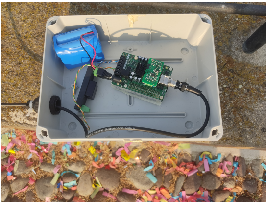
Figure 11: One of the two MODA devices used for the experiment. The board is connected to the battery and to the cable of the hydrophone.
