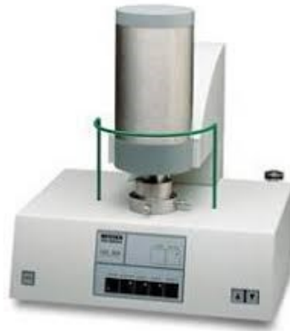
Figure 26: DSC Jupiter -404C from NETZSCH [73].
