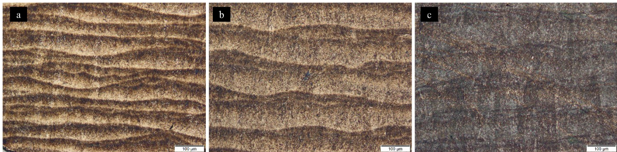
Figure 42: OM micrograph samples post-etching. a) sample treated at 200°C for 10 hours; b) sample treated at 300°C for 10 hours; c) sample treated at 400°C for 10 hours.
