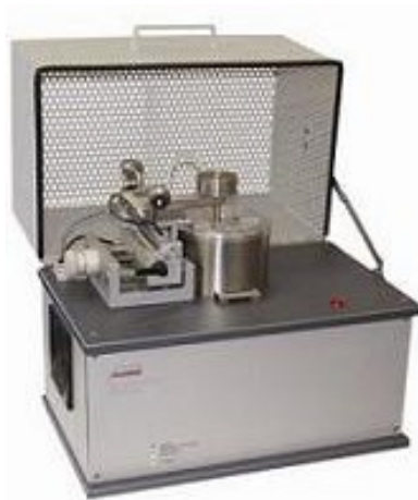
Figure 32: High Temperature Tribometer [77].
