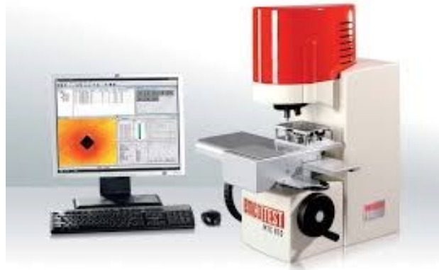
Figure 35: EMCO MIC 010 hardness machine [79].
