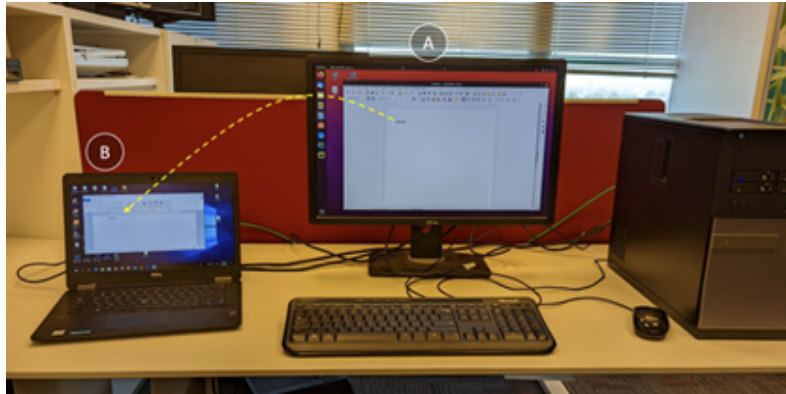
Figure 5.15: SATA cable covert channel
