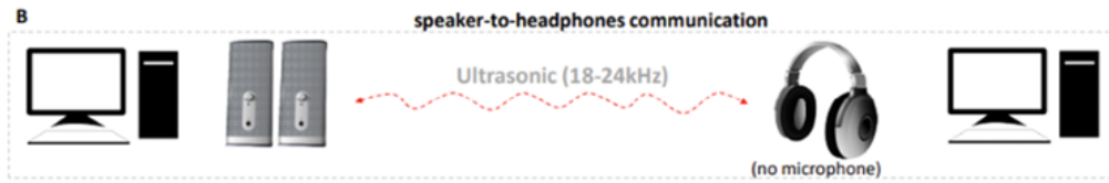
Figure 5.10: Speaker to headphone Cover channels[6]
