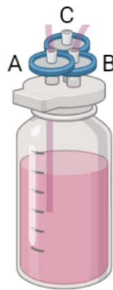
Figure 2.14: reservoir with syringe filters. A) inlet filter; B) outlet filter; C) air filter.
