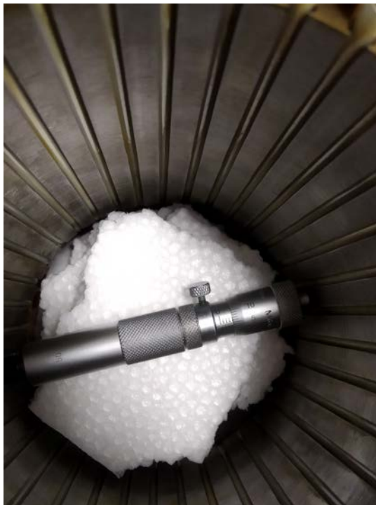
Figure 2.2: Measuring of stator inner diameter
