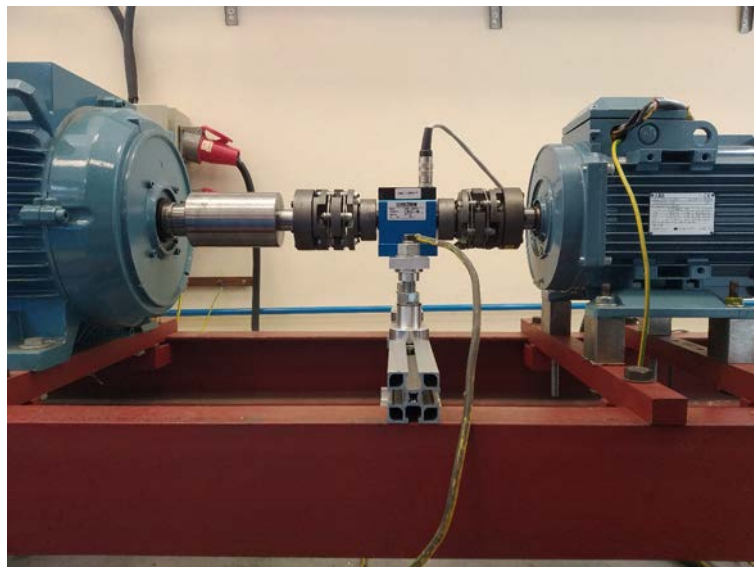
Figure 6.3: Torque sensor and mechanical couplings detail
