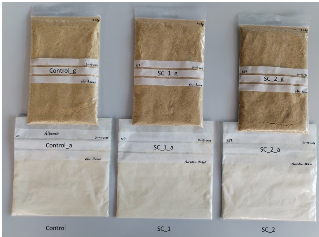
Figure 23. Freeze-dried protein powder of control and fermented samples. Globulin fraction (top) and albumin fraction (bottom).
