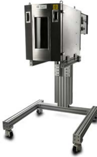
Figura 2.23: Camera climatica MTS 651.05F-01
