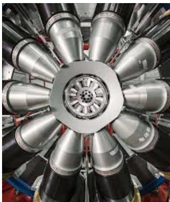
Figure 2.4: Frontal view of Galileo with the ten detectors placed at 90 degrees.
