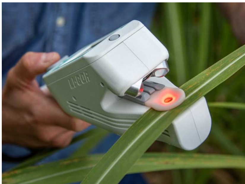
Figure 2.27. Clamp and measurement of the leaf with LI-600 [71].
