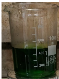
Figure 9. Green-returned solution after adding more ammonia. The iron (III) complexes probably formed are dissolved again as the solution turned at the initial color.
