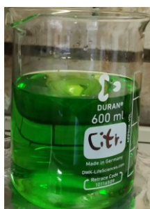
Figure 6. Solution containing cations and citrate. The green color is given by the presence of nickel and iron, probably complexed by the nitrates present; the magnesium in solution is colorless.
