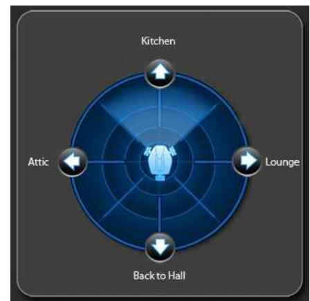
FIGURE 2.3. Controlling a mobile device with four high-level destination commands: three select new destinations, one for going back to last destination
