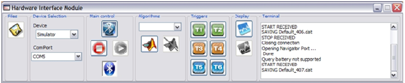
FIGURE 2.10. Main windows of HIM. Starting from the left, user can choose the device for signal acquisition, starting and stopping HIM execution, selects triggers and display plotted results
