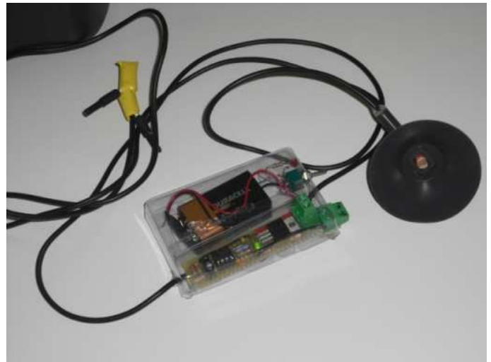
FIGURE 2.15. Blink sensor. The black cap store the photodiode and assure protection against external artifacts.
