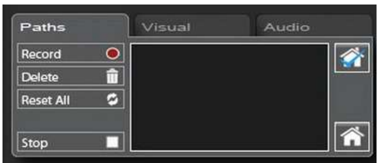
Figure 2.24. (a) A simple real environment schematization for Rovio path management. (b) Path Management form on Rovio Web-based application. Up to 256 paths can be created and stored in Rovio Flash memory. (c) Rovio and its docking station.
