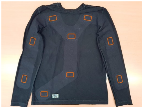
Figure 20 - Sensor shirt with the position of the sensor nodes marked in orange [28]
