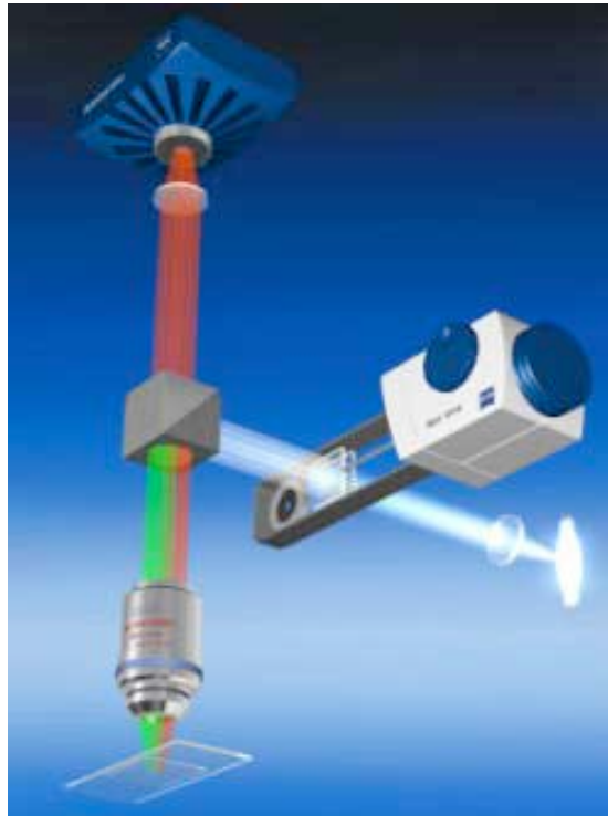
Fig.11 Structured illumination with the ApoTome. The fluorescence excitation light passes through two glass plates in the ApoTome slider. There is a grid structure on the first glass plate; the grid pattern is “imprinted” in the excitation light. The second (plane-parallel) glass plate is tilted by a scanning mechanism, thereby slightly shifting the beam path with the imprinted grid pattern. The excitation light (green) with the grid pattern is then projected onto the specimen via a conventional fluorescence filter set. The emission light (red) is collected by the objective and imaged onto the camera sensor. From Bauch H. et al., 2006.
