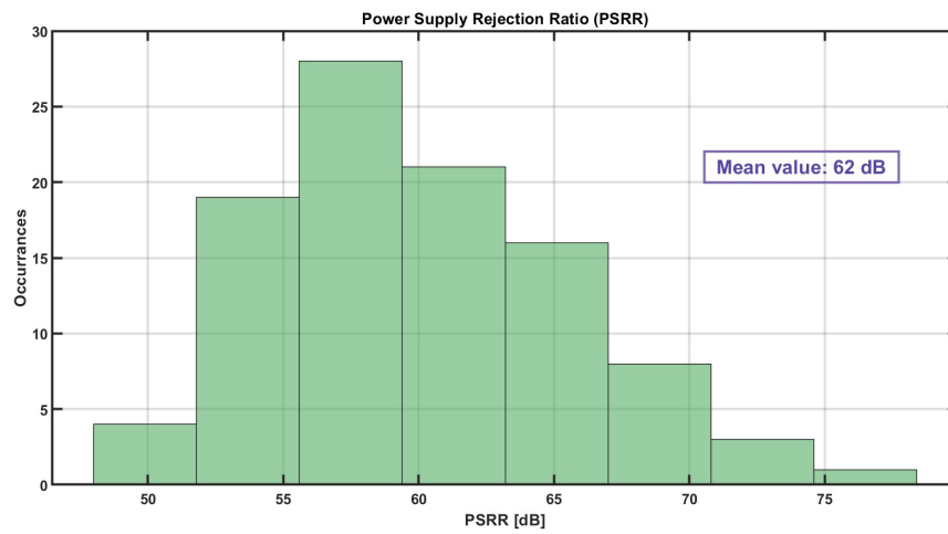
Figure 45: Histogram of the power-supply rejection ratio PSRR of the amplifier, extracted from a Monte Carlo simulation with 100 runs.
