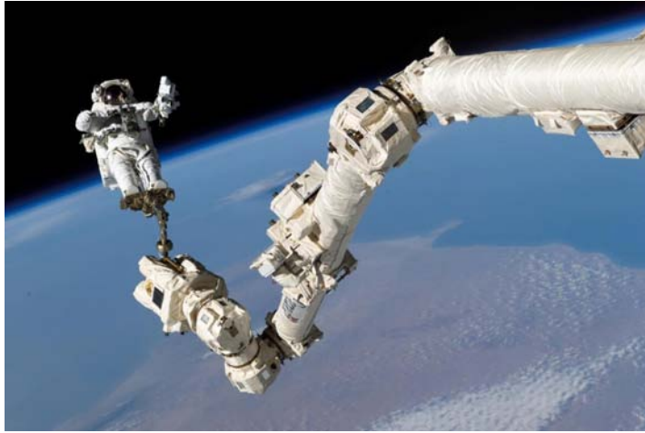
Figure 2.4: An astronaut using a SRMS to work outside the shuttle
