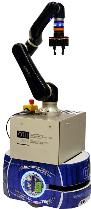
Figure 1.2: Mobile manipulator developed by RRRU.
