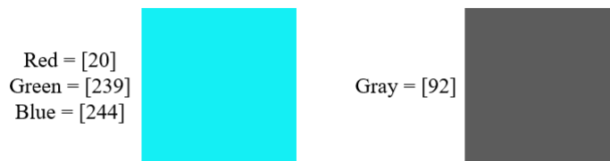
Figure 2.1: Visualization of a RGB pixel versus a gray-scale one
