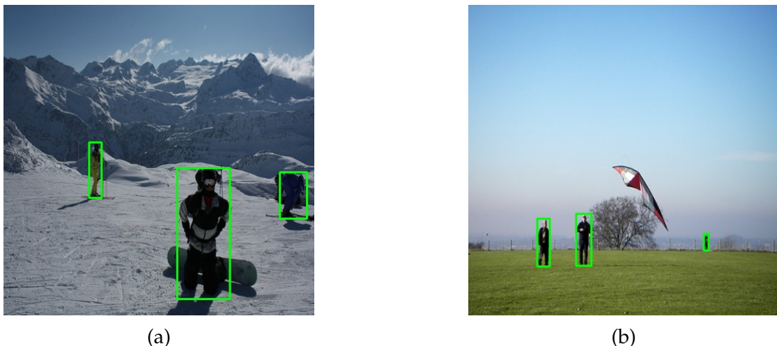
Figure 3.4: Some example images and their ground truths of the Coco dataset regarding the "Person" class, the true bounding boxes are drawn over the images as green rectangles.
