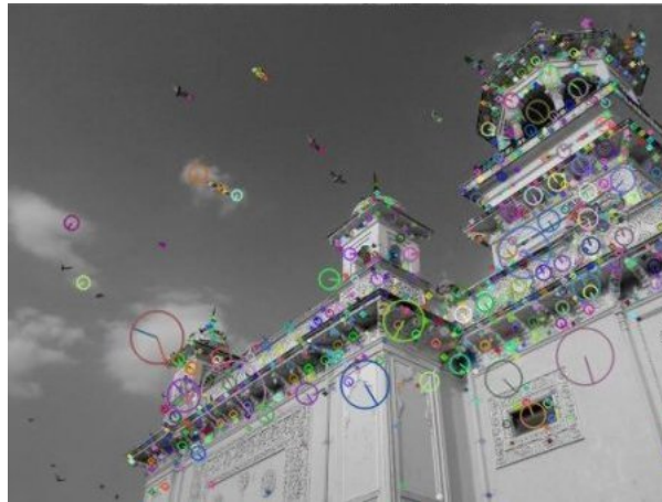
Figure 2.2: Visualization of the popular Sift (Scale Invariant Feature Transform) features
