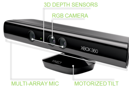
Figure 4.1: Microsoft Kinect sensor illustration
