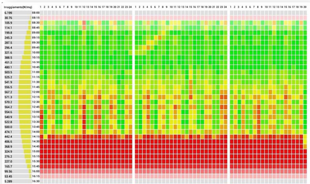
Fig. 5.11 Performance stringhe inverter 3 – 06/01/2012
