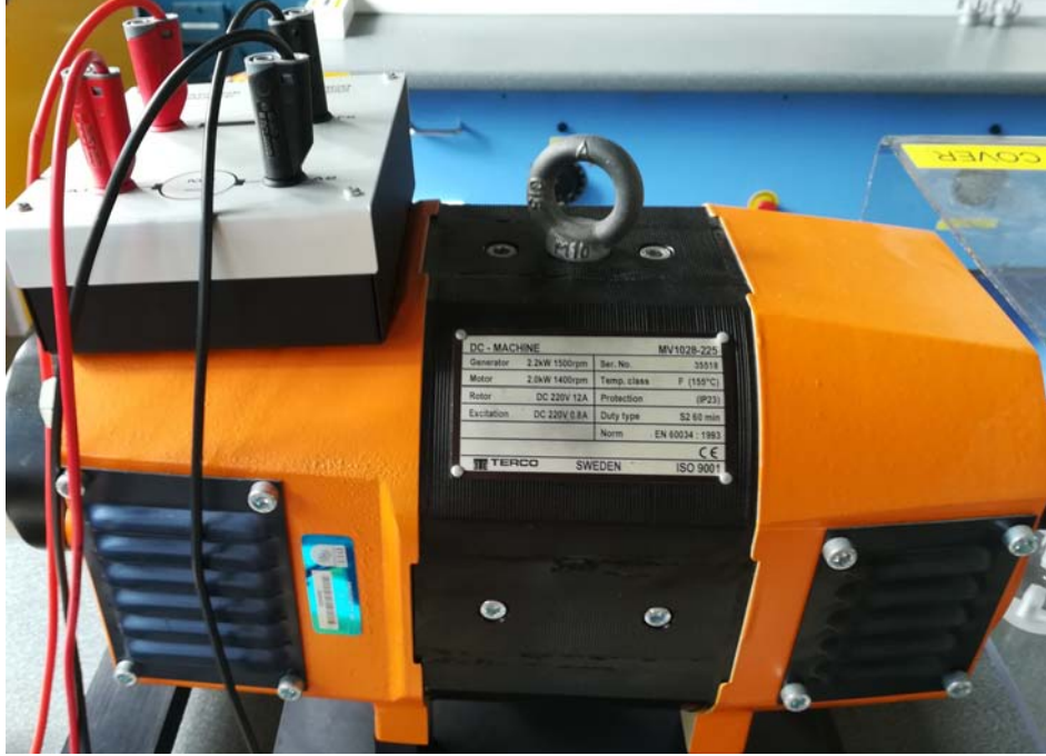
Figure 3.3: DC machine present in the lab and employed in the project as prime mover
