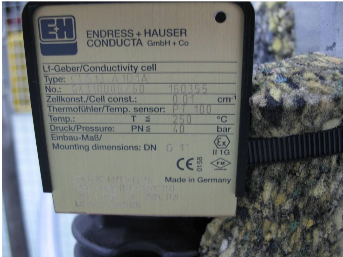
Figure A.8: Particular of sensor cell used, it is possible to see that the constant cell is 0.01 \text{ cm}^{-1} .
