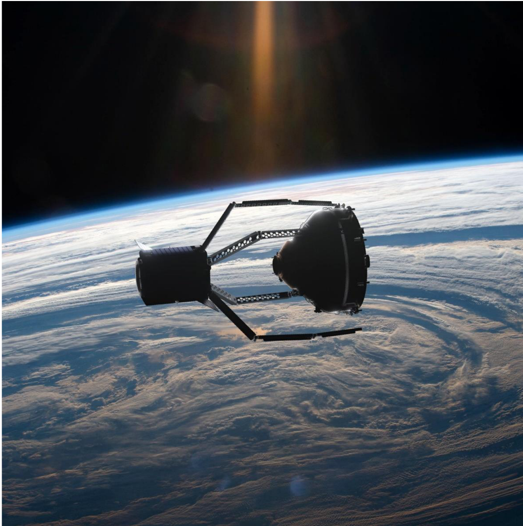
ClearSpace-1 approaching the VESPA module with the four deployed tentacles. Credits: ESA
