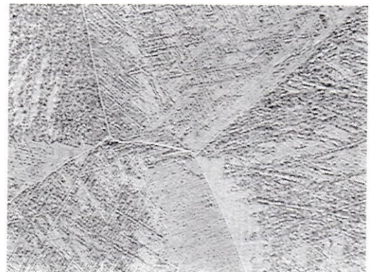
(b) Ti-6Al-4V: Fine lamellar
