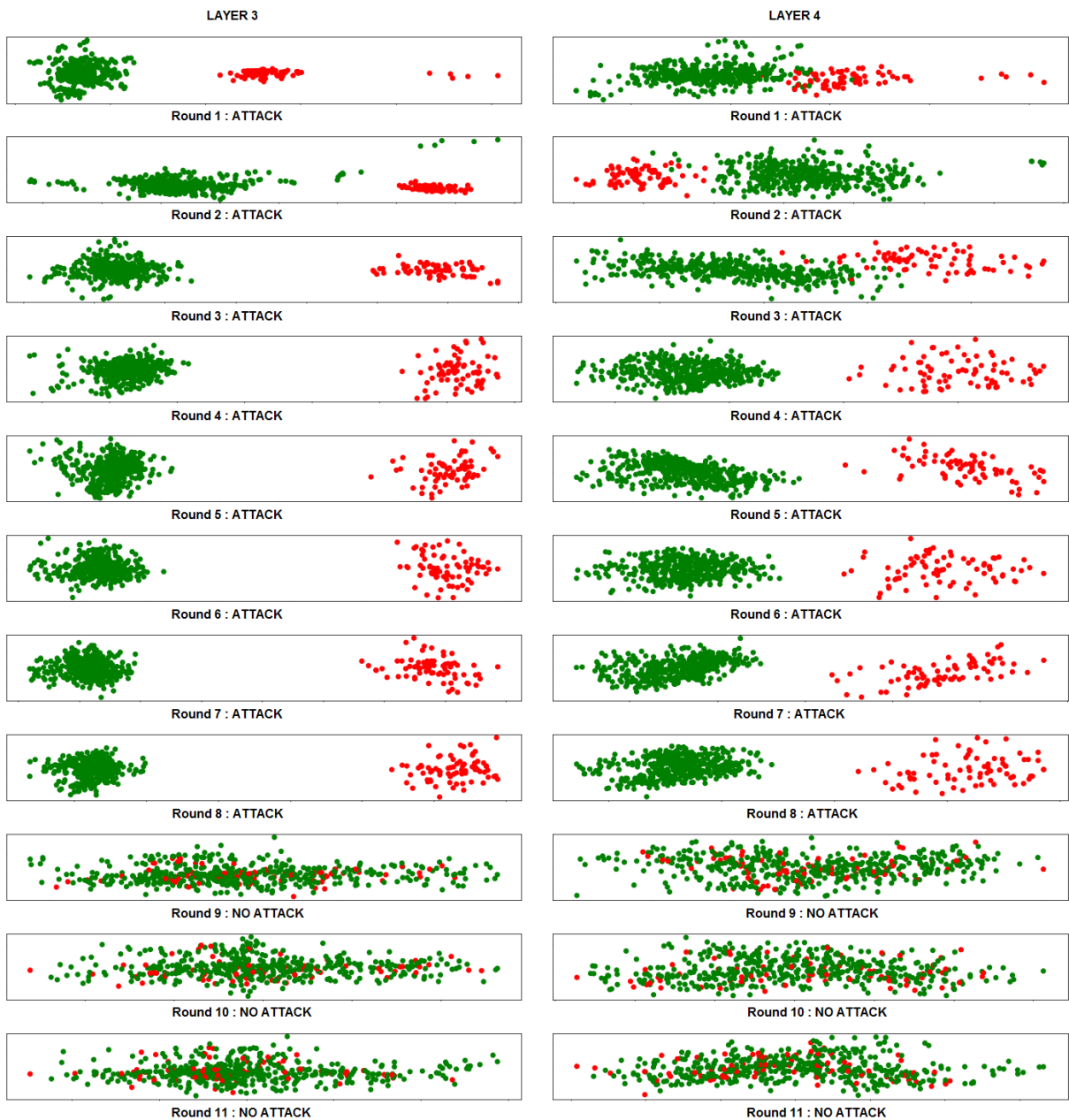
Figure 5.1: Output from the last layer (Layer4) on the right column, output from the Layer3 on the left side, the green dots represent benign models instead red dots are the evils, data are completely IID with 49 evils and 100 clients. Attack presents on the first 8 rounds.
