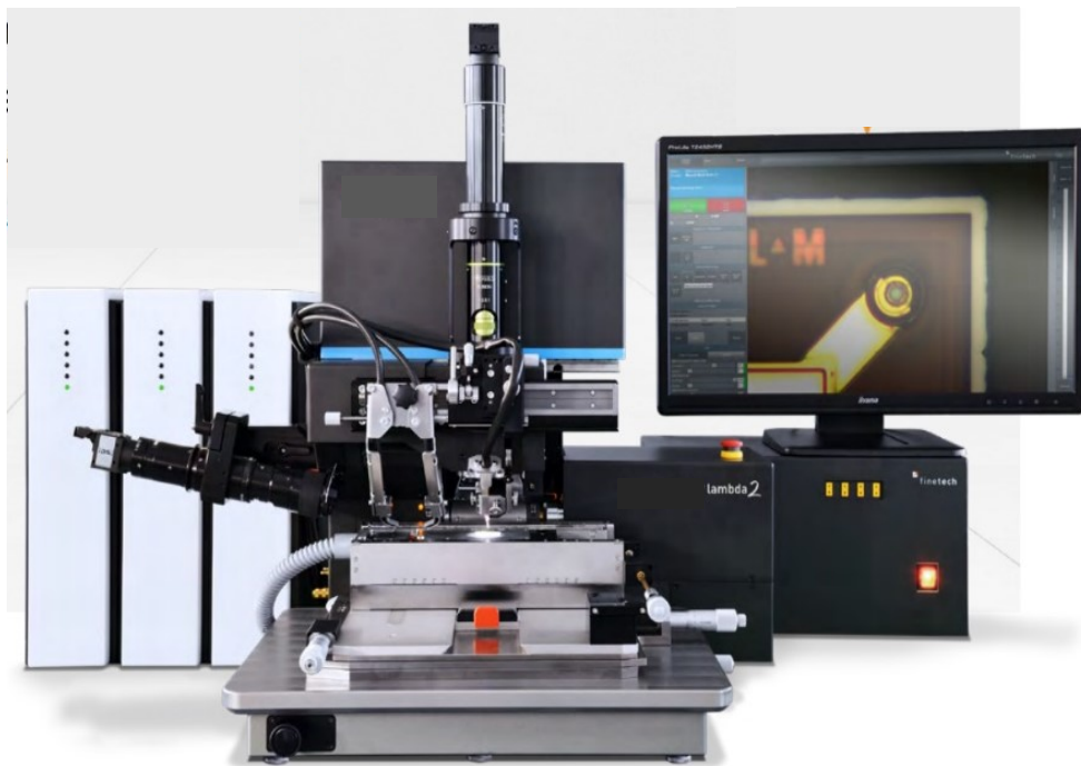
Figure 46 - The machine Lambda with its components
