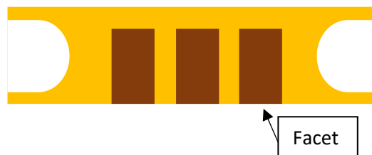
Figure 56 – Representation of CoC mounted on a Heat Sink
