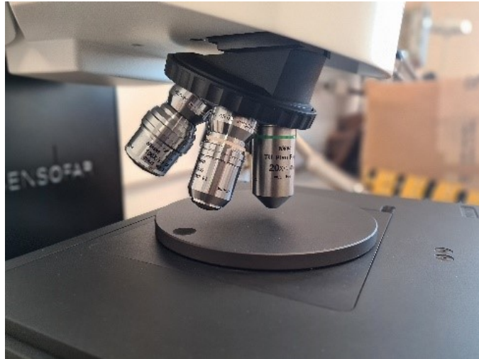
Figure 60 - Sensofar plate where the sample is placed and the lens available by the instrument
