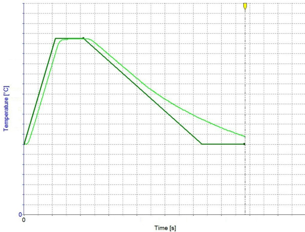
Figure 44 - Example of the temperature ramp used during the CoC assembly process by the Lambda machine. The darker line represents the theoretical ramp while the lighter line represents the ramp performed by the machine in real time
