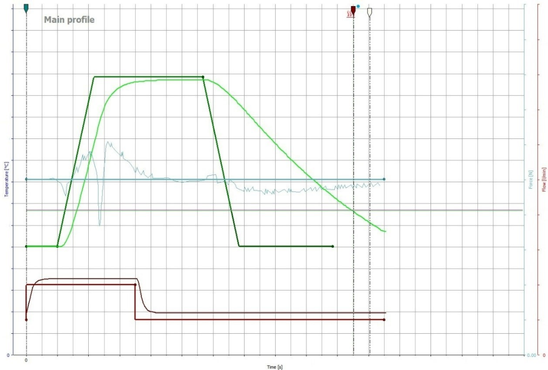
Figure 45 - Example of the temperature ramp used during the CoC assembly process by the Femto2 machine. The darker green line represents the theoretical ramp while the lighter one represents the ramp performed by the machine in real time. Below, in red, there is the representation of the forming gas flow both theoretical and real.
