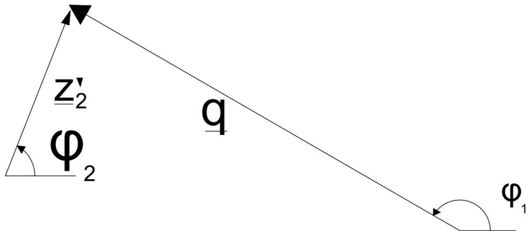
$$\dot{q} \begin{Bmatrix} \cos \varphi_1 \\ \sin \varphi_1 \end{Bmatrix} + q \begin{Bmatrix} -\sin \varphi_1 \\ \cos \varphi_1 \end{Bmatrix} \dot{\varphi}_1 - a'_2 \begin{Bmatrix} -\sin \varphi_2 \\ \cos \varphi_2 \end{Bmatrix} \dot{\varphi}_2 = \begin{Bmatrix} 0 \\ 0 \end{Bmatrix}$$
