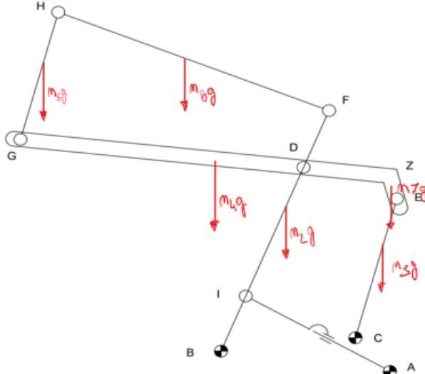
$$\underline{S} = \begin{Bmatrix} -F \\ -m_2g \\ -m_3g \\ -m_4g \\ -m_5g \\ -m_6g \\ -m_7g \end{Bmatrix} \quad \underline{u} = \begin{Bmatrix} q \\ y_{G2} \\ y_{G3} \\ y_{G4} \\ y_{G5} \\ y_{G6} \\ y_{G7} \end{Bmatrix} \quad \underline{w} = \frac{d\underline{u}}{dq} = \begin{Bmatrix} 1 \\ y'_{G2} \\ y'_{G3} \\ y'_{G4} \\ y'_{G5} \\ y'_{G6} \\ y'_{G7} \end{Bmatrix}$$
